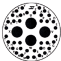
25-42 - 25-42* 38 #20, 4 #8 Coax I, Coax
