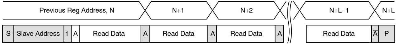
Figure 11. Sequential READ, Start from Current Location
