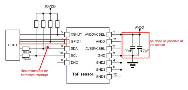
Capacitors on external supply AVDD should be placed as close as possible to the AVDDVCSEL and AVSSVCSEL module pins.
