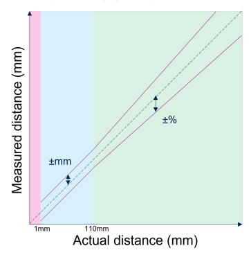
Figure 16. Ranging accuracy vs. distance
