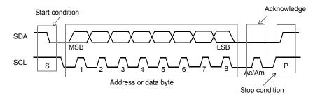
Information is packed in 8-bit packets (bytes) and is always followed by an acknowledge bit, Ac for VL53L4CX acknowledge and Am for controller acknowledge (host bus controller). The internal data is produced by sampling SDA at a rising edge of SCL. The external data must be stable during the high period of SCL. The exceptions to this are start (S) or stop (P) conditions when SDA falls or rises respectively, while SCL is high.
