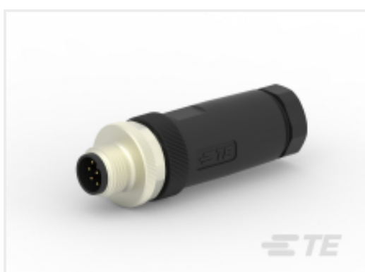
TE Part #T4111001081-000 M12,MALE,STRAIGHT,A CODE,8P, PG7,GOLD
