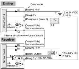
Notes: 1) Input (pink) is the job indicator input when No. 4 of the operation mode switch on the emitter is set to the OFF side, and it is the test input (emission halt input) when the switch is set to the ON side.
