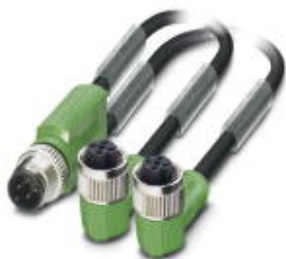
Sensor/actuator cable, 3-position, PUR/PVC, yellow, Plug straight M12, A-coded, on Socket angled M12, A-coded and Socket angled M12, A-coded, cable length: 1 m
