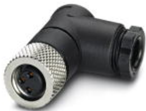
Connector, 3-position, Socket angled M8, A-coded, Solder connection, knurl material: Nickel-plated brass, external cable diameter 3.5 mm ... 5 mm
