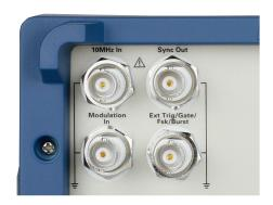
Use the external 10 MHz clock input to synchronize your signals to a master time base. The Sync output generates a TTL pulse for synchronization to a channel's frequency. An external trigger connector is also available for inputting or outputting trigger signals.
