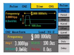
The large 3.5" color display highlights the currently selected channel and shows all relevant parameters with a preview of the waveform being generated.
