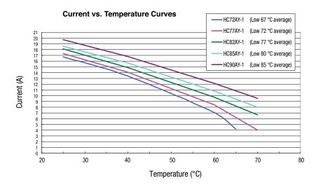
The above curves were derived from placing test samples in an oven at 25 °C, 40 °C, 60 °C and 70 °C, increasing current flow through the sample at a rate of 0.1 A/minute and recording the current value when the sample trips.
