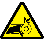
W3154 Belt Drive Entanglement Hazard
