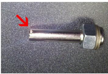
2) At the bottom of the bolt you will notice a small screw. Remove screw and save.
