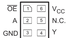
Figure 5-1. DBV package 5-pin SOT-23 (Top View)
