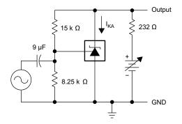
Figure 15. Test Circuit for Voltage Amplification
