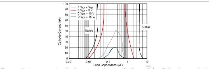
The areas under the curves represent conditions that may cause the device to oscillate. For curves B, C, and D, R2 and  $V_{REF}$  were adjusted to establish the initial  $V_{KA}$  and  $I_{KA}$  conditions with  $C_L = 0$ .  $V_{BATT}$  and  $C_L$  then were adjusted to determine the ranges of stability (see Figure 18 and Figure 19 for test circuits).
