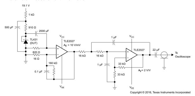
Figure 14. Test Circuit for Equivalent Input Noise Voltage
