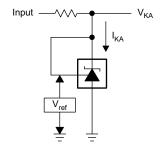
Figure 20. Test Circuit for  $V_{KA} = V_{REF}$
