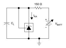
Figure 18. Test Circuit for Curve A
