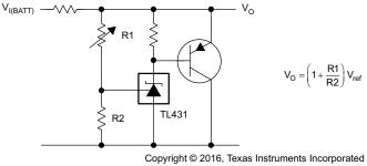
Figure 32. High-Current Shunt Regulator
