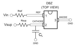
Figure 41. DBZ Layout Example
