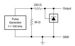
Figure 17. Test Circuit for Pulse Response
