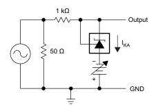
Figure 16. Test Circuit for Reference Impedance
