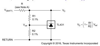
A. R must provide cathode current  $\geq$ 1 mA to the TL431-Q1 at minimum  $V_{I(BATT)}$ .
