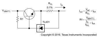
Figure 39. Precision Current Limiter
