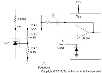
Figure 36. PWM Converter with Reference
