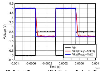
Figure 27. Output Response With Various Cathode Currents
