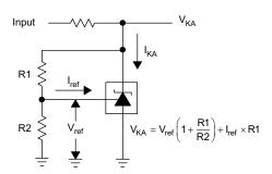
Figure 21. Test Circuit for  $V_{KA} > V_{REF}$
