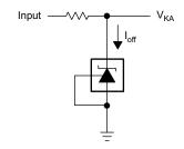
Figure 22. Test Circuit for I<sub>OFF</sub>
