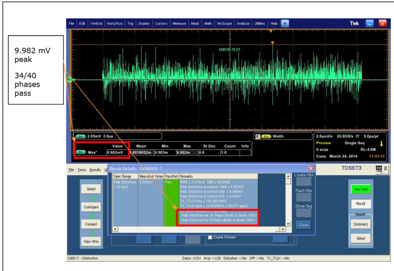
FIGURE 5: ETHERNET COMPLIANCE REPORT FOR LESS THAN 100% OF THE UI PASSING
