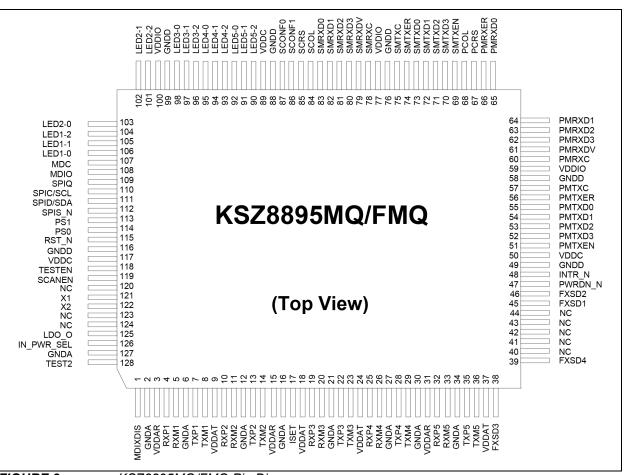
FIGURE 2: KSZ8895MQ/FMQ Pin Diagram.
