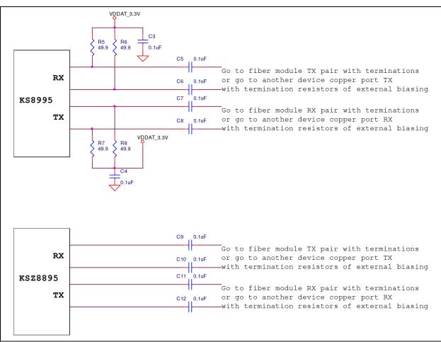
FIGURE 4: Connection Comparison for Fiber Module or Cap AC-Coupling with Two Copper Ports.
