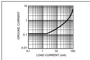
FIGURE 2-1: Ground Pin Current vs. Load Current.
