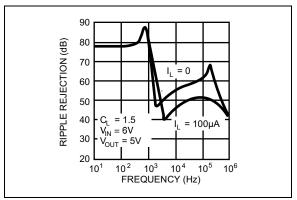
**FIGURE 2-23:** Power Supply Ripple Rejection.
