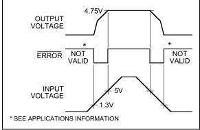
FIGURE 4-1: ERROR Output Timing.
