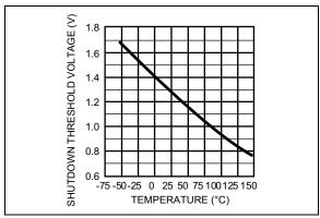
**FIGURE 2-28:** Shutdown Threshold Voltage vs. Temperature.
