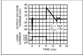
FIGURE 2-20: Load Transient Response.
