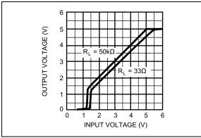
FIGURE 2-2: Dropout Characteristics.
