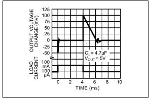
FIGURE 2-19: Load Transient Response.
