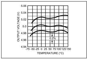
FIGURE 2-5: Output Voltage vs. Temperature of 3 Representative Units.
