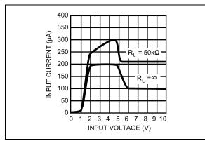
**FIGURE 2-3:** Input Current vs. Input Votlage.
