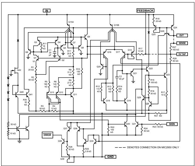
FIGURE 5-1: Schematic Diagram.
