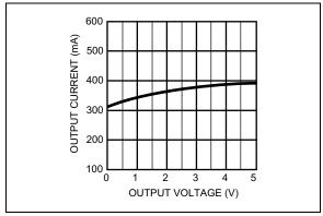
FIGURE 2-32: Foldback Current Limiting.
