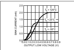
FIGURE 2-17: Comparator Sink Current vs. Output Low Voltage.
