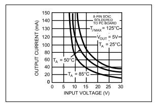
**FIGURE 2-30:** Maximum Rated Output Current vs. Input Voltage.
