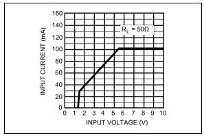
FIGURE 2-4: Input Current vs. Input Voltage.
