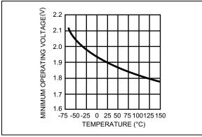
**FIGURE 2-13:** Minimum Operating Voltage vs. Temperature.
