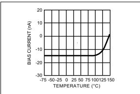
FIGURE 2-14: Feedback Bias Current vs. Temperature.
