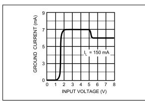
FIGURE 2-9: Input Voltage.
