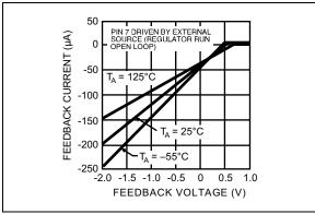
FIGURE 2-15: Feedback Pin Current vs. Feedback Voltage.
