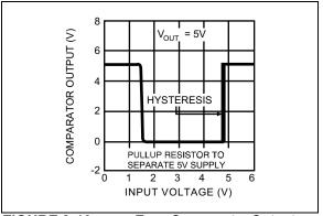
FIGURE 2-16: Error Comparator Output vs. Input Voltage.
