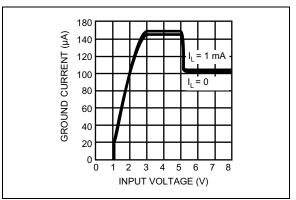
**FIGURE 2-6:** Ground Pin Current vs. Input Voltage.
