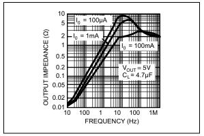
FIGURE 2-22: Output Impedance.
