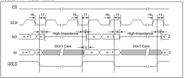
FIGURE 1-2: SERIAL INPUT TIMING
