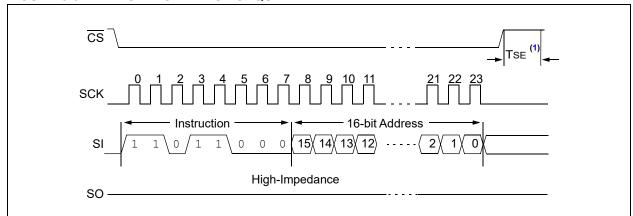
Note 1: This sequence initiates a self-timed internal write cycle on the rising edge of CS after a valid sequence.
