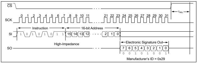
Driving  $\overline{\text{CS}}$  high after the 8-bit RDID command but before the Electronic Signature has been transmitted will still ensure the device will be taken out of Deep Power-Down mode, as shown in Figure 3-13.
