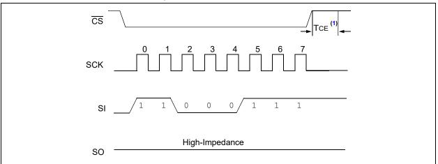
Note 1: This sequence initiates a self-timed internal write cycle on the rising edge of CS after a valid sequence.
