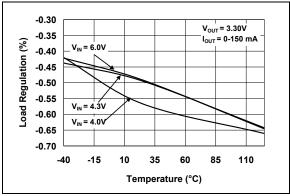
*FIGURE 2-8:* Load Regulation vs. Temperature.
