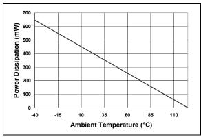
FIGURE 5-3: Power Dissipation vs. Ambient Temperature (SOT-23 Package).
