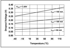
*FIGURE 2-10:* Dropout Voltage vs. Temperature.
