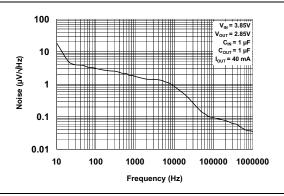
FIGURE 2-17: Output Noise vs. Frequency.
