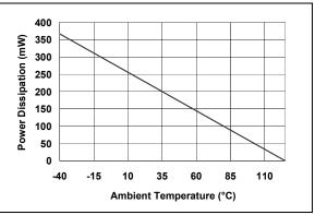
FIGURE 5-1: Power Dissipation vs. Ambient Temperature (SC-70 package).
