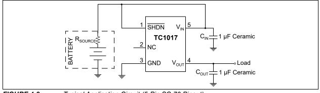
FIGURE 4-2: Typical Application Circuit (5-Pin SC-70 Pinout).
