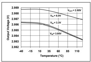
*FIGURE 2-16:* Output Voltage vs. Temperature.
