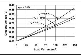
FIGURE 2-1: Dropout Voltage vs. Output Current.
