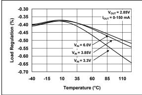
**FIGURE 2-2:** Load Regulation vs. Temperature.
