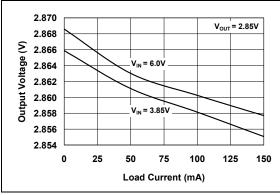
FIGURE 2-13: Output Voltage vs. Output Current.
