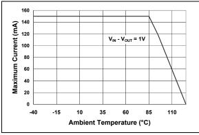
FIGURE 5-4: Maximum Current vs. Ambient Temperature (SOT-23 Package).
