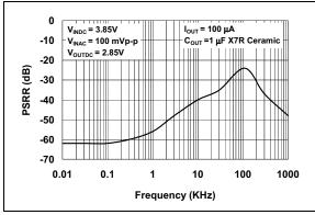
*FIGURE 2-15:* Power Supply Rejection Ratio vs. Frequency.
