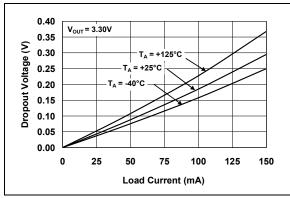
FIGURE 2-7: Dropout Voltage vs. Output Current.
