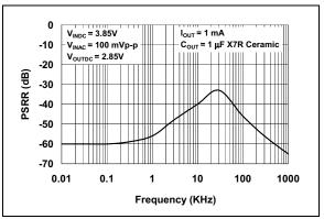
FIGURE 2-18: Power Supply Rejection Ratio vs. Frequency.
