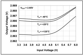
FIGURE 2-12: Output Voltage vs. Supply Voltage.
