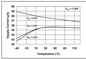
*FIGURE 2-9:* Supply Current vs. Temperature.
