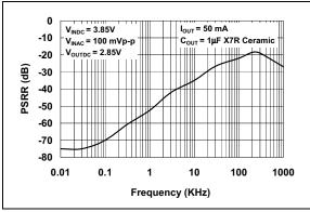
*FIGURE 2-19:* Power Supply Rejection Ratio vs. Frequency.
