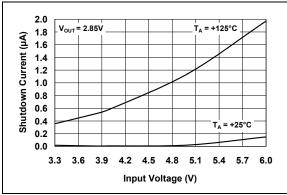
FIGURE 2-14: Shutdown Current vs. Input Voltage.
