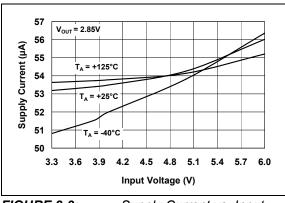
FIGURE 2-3: Supply Current vs. Input Voltage.
