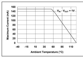
FIGURE 5-2: Maximum Current vs. Ambient Temperature (SC-70 package).
