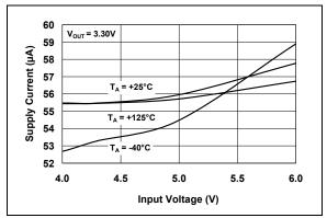
FIGURE 2-11: Supply Current vs. Input Voltage.
