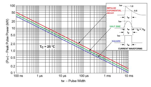
Figure 4-1. Peak Pulse Power Vs. Pulse Time
