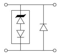
Figure 6-3. Optional Bidirectional Configuration (Two TVS Devices in Anti-Parallel)
