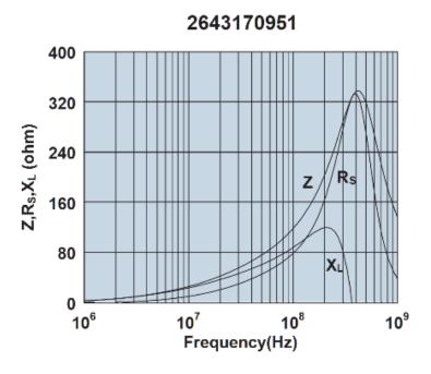
Impedance, reactance, and resistance vs. frequency.
