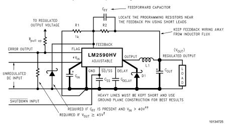
Select  $R_1$  to be approximately 1  $k\Omega$ , use a 1% resistor for best stability.
