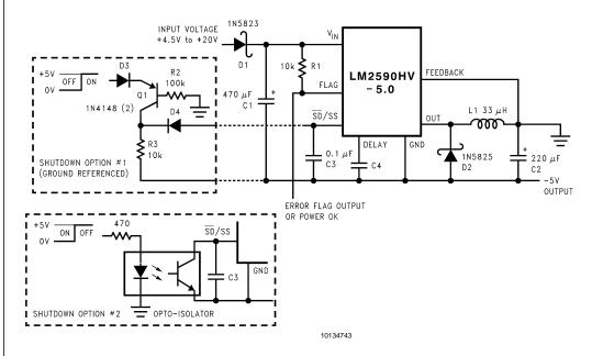
FIGURE 10. Inverting -5V Regulator With Shutdown and Soft-start
