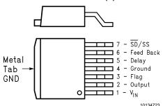
Order Number LM2590HVS-3.3, LM2590HVS-5.0, or LM2590HVS-ADJ See NS Package Number TS7B
