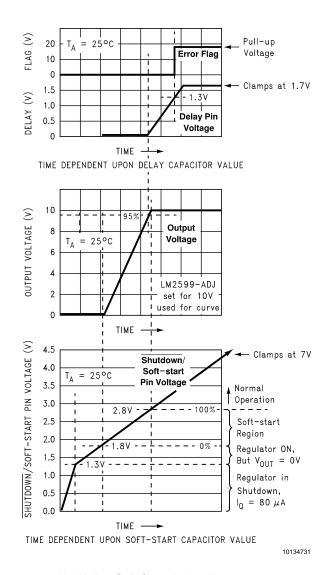
FIGURE 2. Soft-Start, Delay, Error Output
