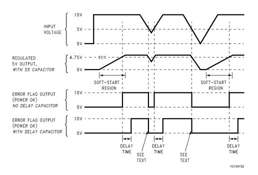
FIGURE 3. Timing Diagram for 5V Output
