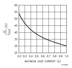
FIGURE 7. Current Ripple Ratio
