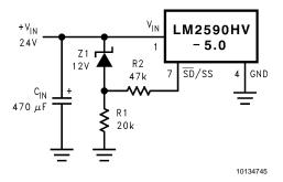
FIGURE 11. Undervoltage Lockout for a Buck Regulator
