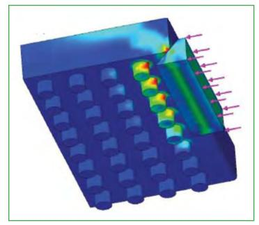
Figure 4. von Mises Stress Plot for BGA with maxiGRIP<sup>™</sup> Frame Clip Installed.
