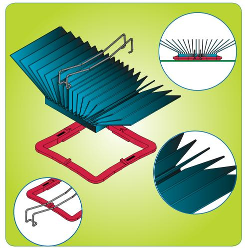
Figure 1. The maxiGRIP Heat Sink Assembly.
