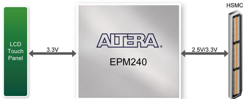
Figure 3-6 Block Diagram of the Bus Controller
