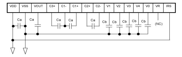
4.2.2. When using the internal power supply circuit (except voltage booster circuits) (In case of V0 voltage external regulator resistors)
