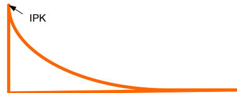
Figure 47. Input Charge Inrush Current
