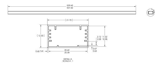
Figure 47: Tube Design for Rectangular Array Products
