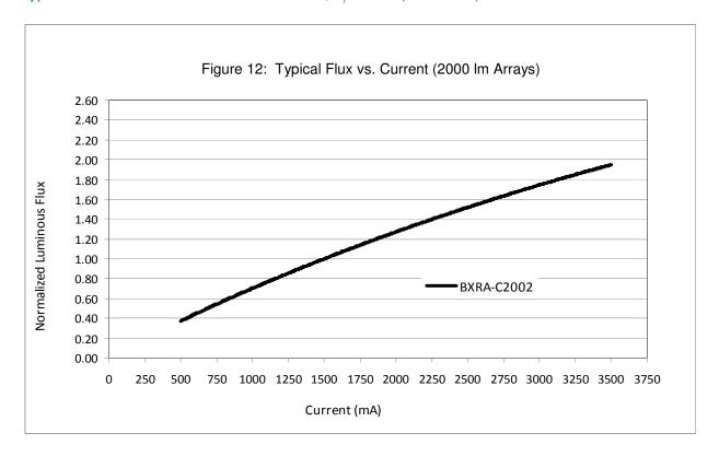
Note for Figures 8 through 12: Bridgelux does not recommend driving high power LED Arrays at low currents. Doing so may produce unpredictable results. Pulse width modulation (PWM) is recommended for dimming effects.
