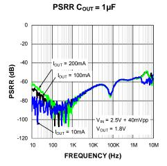
Figure 1. MIC94310 Ripple Blocker™ **Frequency Response**
