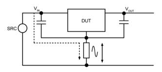
Figure 2. High-Frequency Noise on **Measurement System**
