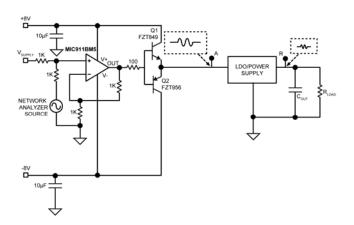
Figure 3. Network Analyzer Set-Up
