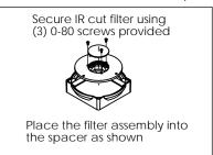
NOTE: Filter Holder cannot be used with CS Adaptor
