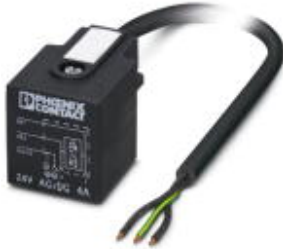
Sensor/Actuator cable, 3-position, PVC, Black RAL 9005, Free cable end, on A valve plug, with 1 LED, connected with Z diode, Cable length: 10 m
