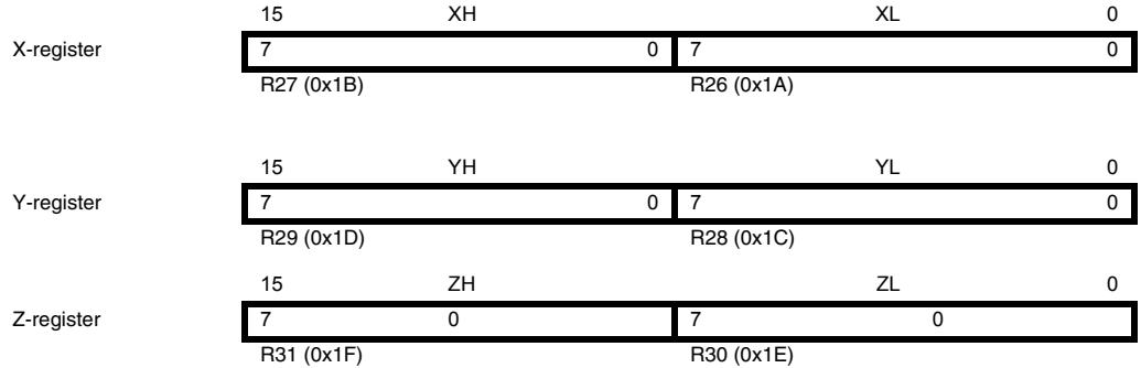
Figure 5. The X-, Y-, and Z-registers
