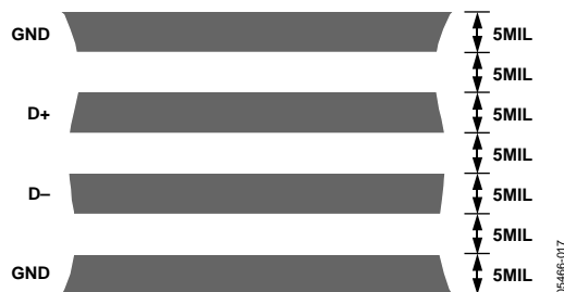
Figure 22. Typical Arrangement of Signal Tracks
