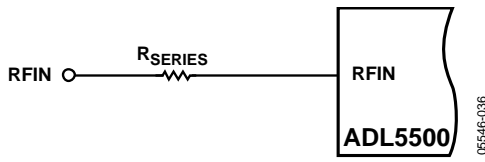
Figure 36. Attenuating the Input Signal
