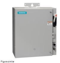
Pump control panel, Size 1, Three phase full voltage, Solid-state overload relay, OLR amp range 3-12A, 190-220/220-240V 50/60Hz coil, Standard type contactor, 30A fusible disconnect, 30A/600V fuse clip, HOA Sel Sw. <(>&<)> Start P.B., Enclosure NEMA type 3/3R, Weather proof outdoor use
