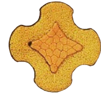
4 points shape cross section turned contact
