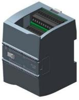
SIPLUS S7-1200 SM 1223 16DI/16DQ based on 6ES7223-1BL32-0XB0 with conformal coating, -40...+70 °C, start up -25 °C, digital input/output 16 DI/16 DQ, 16 DI 24 V DC, sink/source, 16 DQ, transistor 0.5 A
