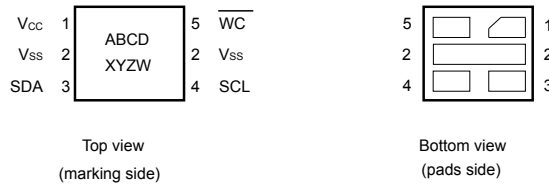
Figure 3. UDFPN5 (DFN5) package connections
