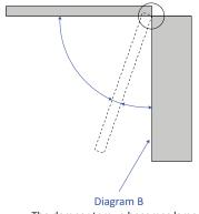
The damper torque becomes larger, preventing the lid from closing completely
