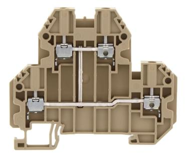
Double-level terminal, Screw connection, Mounting type: Mounting rail TS 35/7.5, Rated cross-section: 2.5 mm<sup>2</sup>, Width: 5.1 mm, Colour: Beige
