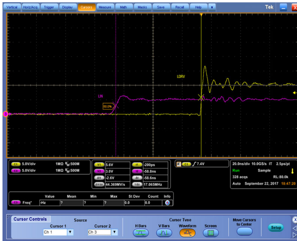
Figure 30. Low Side Turn-ON Propagation Delay (NCP51530A)
