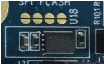
Figure 17: Optional external serial SPI flash IC (U18) schematic and PCB
