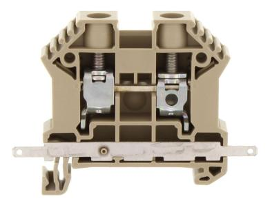
Feed-through terminal, Screw connection, Mounting type: Mounting rail TS 35/7.5, Rated cross-section: 16 mm<sup>2</sup>, Width: 10 mm, Colour: Beige
