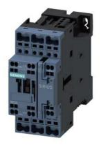
power contactor, AC-3 17 A, 7.5 kW / 400 V 1 NO + 1 NC, AC (50-60 Hz) DC operation 21-28 V AC/DC, 3-pole, Size S0, Spring-type terminal
