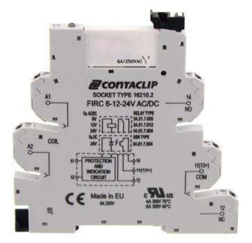
Interface-Relay-Compact (IRC) Complete, Consisting of base FIRC... with Push-In connection and pluggable miniature relay with power contact, Mounting type: Mounting rail TS 35, 1 CO contact, Input voltage: 24 VAC/DC
