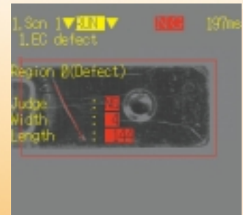
Detects scratches on metal surfaces, even with low-contrast images.
