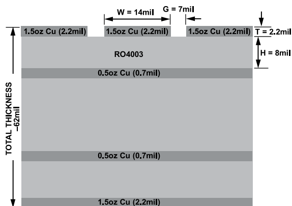
Figure 22. Probe Matrix Board (Cross Section View)
