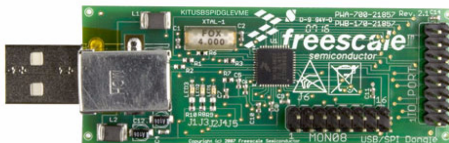
Figure 2. KITUSBSPIDGLEVME Interface Dongle
