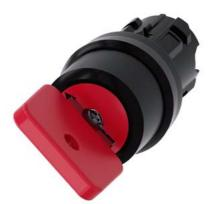
Key-operated switch O.M.R, 22 mm, round, plastic, lock number 73037, red, with 2 keys, 2 switch positions O-I, latching, actuating angle 90°, 10:30h/13:30h, key removal O, with laser labeling, inscription or symbol Customer-specific selection with SIRIUS ACT configurator (CIN)
