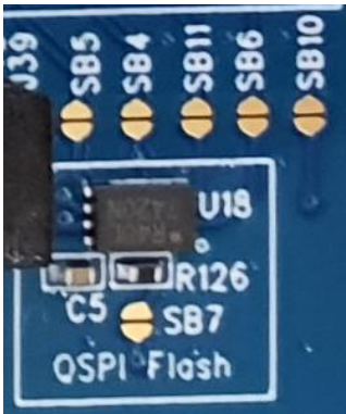
Figure 19: Optional external serial SPI flash IC (U18) schematic and PCB
