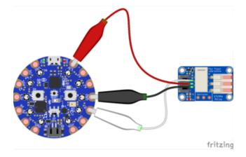
Plug the 3-pin JST to alligator clip cable into the 3-pin JST connector on the STEMMA Relay
