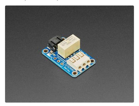
Each STEMMA board comes with a fully assembled and tested PCB but no cable. No soldering is required to use it. There's an optional second switch on the side of the PCB, if you get a 3-pin terminal block () you can solder that in place, but its optional.
