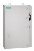
Non-reversing motor starter, Size 2 1/2, Three phase full voltage, Solid-state overload relay, OLR amp range 25-100A, 24VAC 50-60Hz coil, Combination type, 100A non-fusible disconnect, Encl NEMA type 4X 304 S-Steel, Water/dust tight noncorrosive, Extra-wide enclosure
